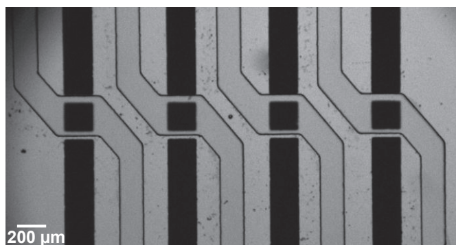
Fig. 2. Image of the microfluidic network for peptide immobilization. Microchannels, 200 μm in width, expand to 300 μm when passing over the middle electrodes of the sensors. Sensors are shown in black.
