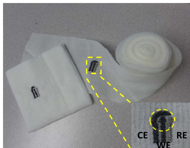
Figure 2: Embroidered electrochemical sensors on medical gauze and wound dressing. Inset shows a close-up view of the sensor.
