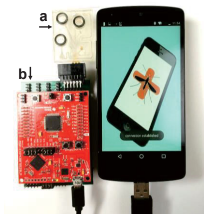
Figure 3: Photograph of our mobile phone biosensing platform. The microfluidic chip (a) directly plugs into aMEASURE (b), which is connected to the phone via the microUSB port using a USB OTG adapter.
